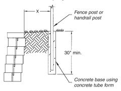
When there is not enough room to set fence posts behind walls, they can be installed within top wall units prior to backfilling behind the wall. Break off the backs of the top few units to create room for the post. Cut or core the cap units to neatly receive posts (Figures 2 and 3). The fence should be flexible enough to accommodate differential movement between the units and the fence.
